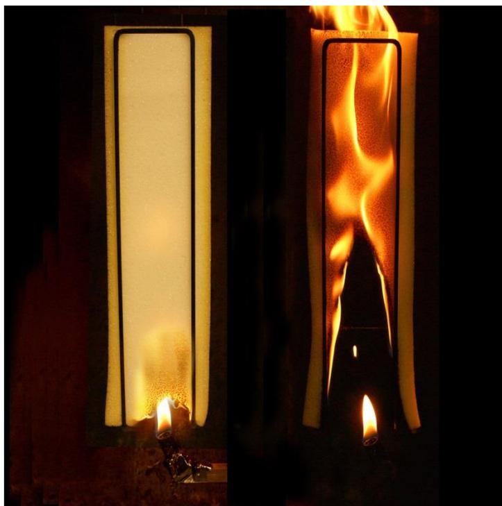
Flame retarded foam (left) and untreated foam (right) in vertical ignition resistance test.
