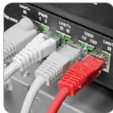
Connectors (PBT, Polyamides)
